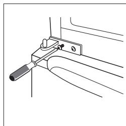
11. Place the upper door back on. Ensure the door is aligned horizontally and vertically so that the seal are closed on all sides before finally tightening the top hinge. Then inert the top hinge and screw it to the top of unit and then fix hinge cover (in accessory bag) by screw.
