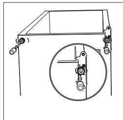
8. Unscrew and remove the bottom hinge pin, turn the bracket over and replace it.
