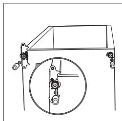
10. Make the middle hinge reverse the direction  $180^\circ$ , then transfer it to the left property position. Make the middle hinge pin in the upper hole of the lower door, then tight the bolts.
