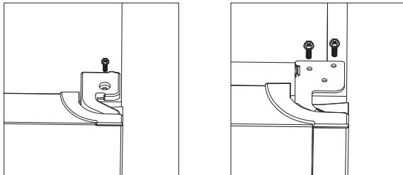
2. Remove the pin with a screwdriver and flip the hinge bracket. Then refit the pin to hinge bracket.
