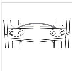
7. Unscrew bottom hinge. Then remove the adjustable feet from both side.
