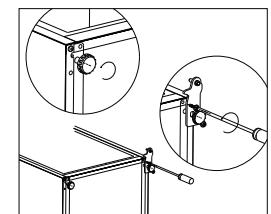
8. Unscrew and remove the bottom hinge pin, turn the bracket over and replace it.
