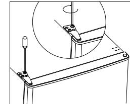
14. Clap in the hinge cover and hole cover on the top of unit.
