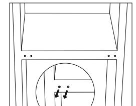
7. Lie down the rear of cabinet on a soft pad. And unscrew the bottom hinge and leveling foot.
