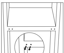
11. Stand up the unit and put the door on the bottom hinge. Make sure the bottom hinge core is inserted in the door hole. Then move the hinge hole cover of bottom door from left side to right side.
